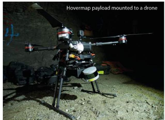
Hovermap payload mounted to a drone
