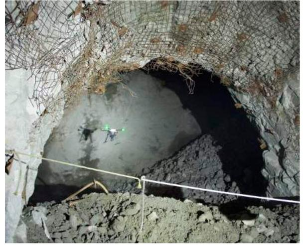
Autonomous flight into a stope
